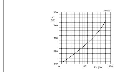
Fig.2 Typical capacitance as a function of relative humidity.
